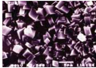
Fig.4: SEM micrograph of modified smear layer with Prisma Universal Bond 2. Samples were demineralized and deproteinized.
